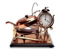
The teasmade designed by Albert (top picture) set up ready for making the tea (bottom picture) after the alarm has gone off ready to pour the water into the waiting teapot.
